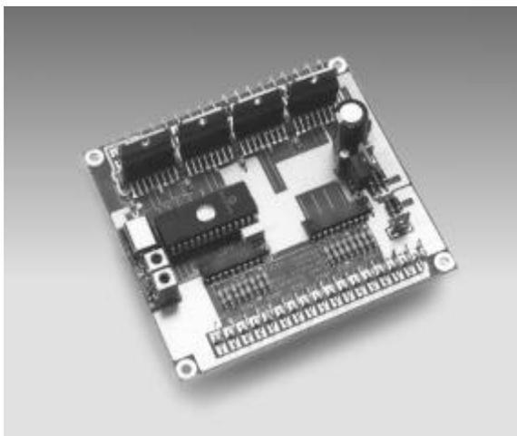
**KAR-108T Accessory Receiver controls up to eight twin coil switch machines.**
