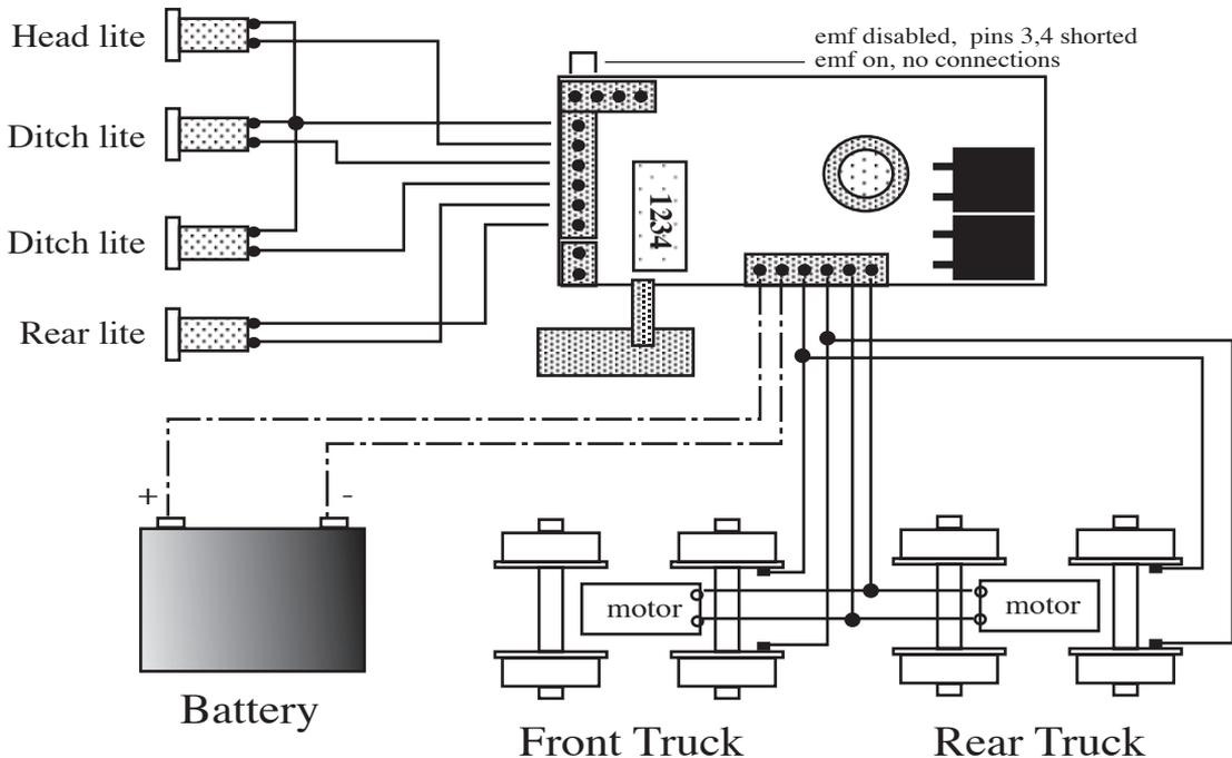
**Warning:** make sure the motor is isolated from all track wiring.
